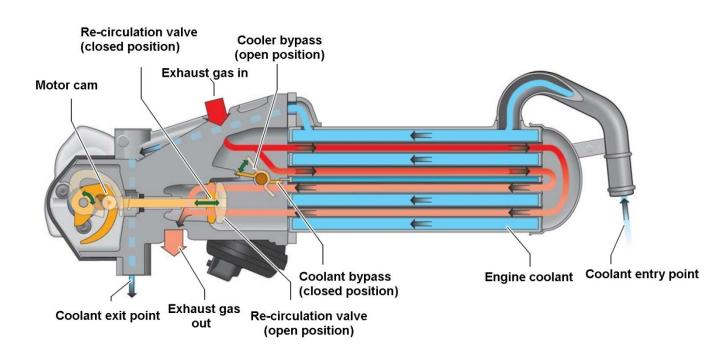
The above diagram shows the functionality of this type of EGR valve
